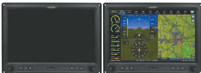
G3X Touch Full-Screen Reversionary Mode (Failed PFD)
