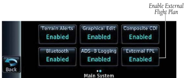
External Flight Plan Enabled (Configuration Mode)
