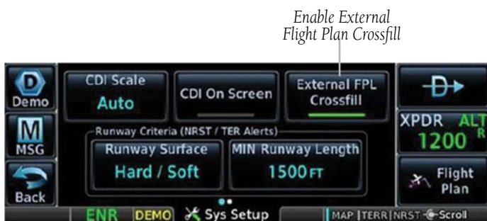
External Flight Plan Crossfill Enabled (Normal Mode)
