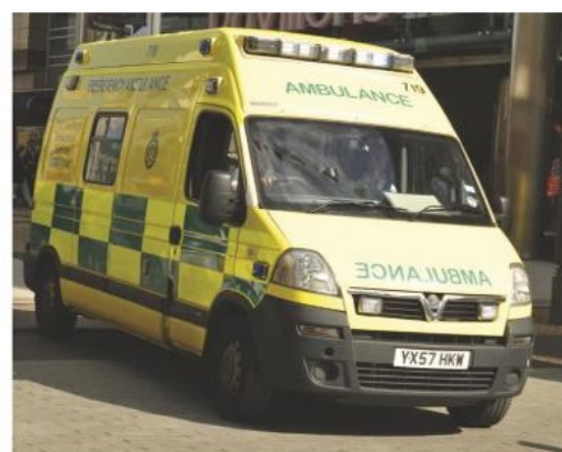
Figure 4 Ambulances and police cars often carry a mirror image sign on the front. This is so the driver of a vehicle in front can read the sign when they look in their mirror because it gets laterally inverted (back to front but not upside down)
