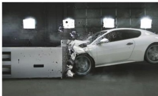
Figure 1 A crash test. Car makers test the design of a crumple zone by driving a remote control car into a brick wall
