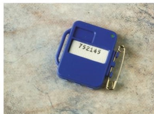
Figure 3 A film badge tells you how much ionising radiation the wearer has received
