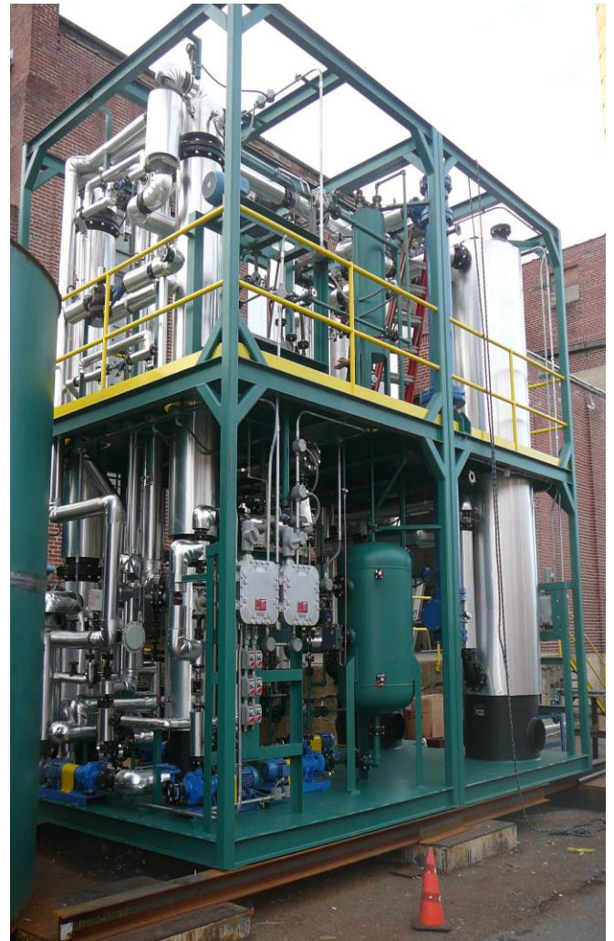
Summit Foods Distillation System and Molecular Sieve
