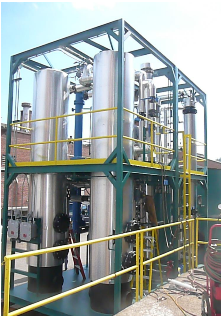
Summit Foods Distillation System and Molecular Sieve
