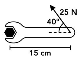
18. A force is applied to a wrench as shown on the right. What is the torque produced by the force, and is it positive or negative?
