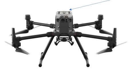
Additional Part 107.29 compliant LEDs groups, which consist of 4 cree LEDs housed in one unit, have been affixed to the top hull portion the sUAS. Each of these LED groups exceed the 3SM visibility requirement and have the ability to strobe, flash, or provide continuous light. Each unit weighs approximately 6 grams, thus not interfering with the sUAS flight dynamics.
