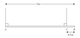
A beam AB has length 5m and mass 25kg. The beam is suspended in equilibrium in a horizontal position by two vertical ropes. One rope is attached to the beam at A and the other rope is attached to the point C on the beam where CB = 0.5m, as shown in Figure 3. A particle P of mass 60kg is attached to the beam at B and the beam remains in equilibrium in a horizontal position. The beam is modelled as a uniform rod and the ropes are modelled as light strings.
