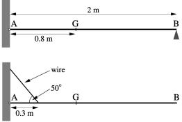
The forces acting on the beam at A due to the hinges are a horizontal force X N in the direction AB, and a downward vertical force Y N, which have a resultant of magnitude R at  $\alpha$  to the horizontal. c. Calculate X, Y, R and  $\alpha$
