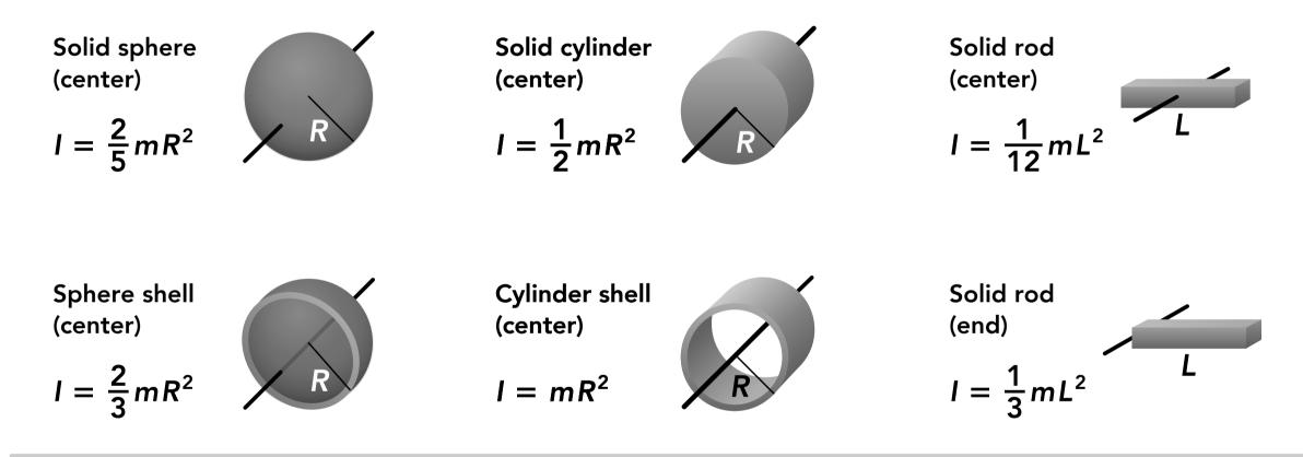
• Since the rotational inertia of an object or system depends on how far the mass is from the axis of rotation, the rotational inertia will change if we move the axis of rotation.
