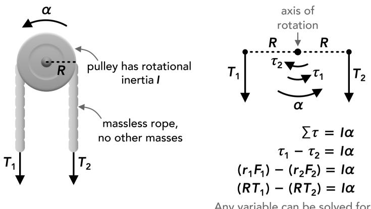
Note: If there were other objects attached to the ropes they would also have mass and their own inertia, and the angular acceleration of the pulley would also depend on the linear dynamics of those masses and the rope.
