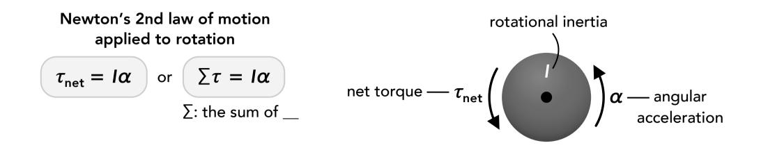
The net torque is the sum of all of the torques acting on an object
