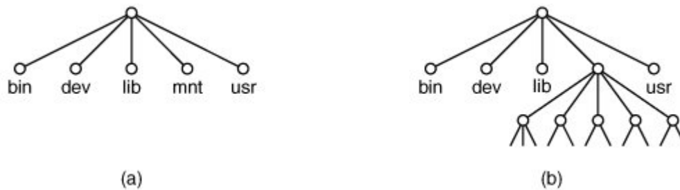
Figure 1-15. (a) File system before the mount. (b) File system after the mount.
