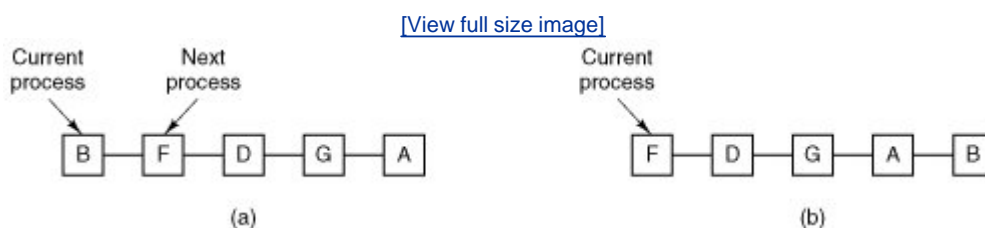
Figure 2-26. Round-robin scheduling. (a) The list of runnable processes. (b) The list of runnable processes after B uses up its quantum.
