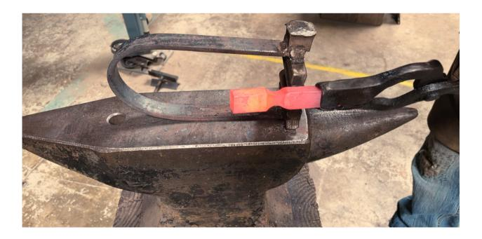
Step 3: From the shoulders created by the fuller, Draw out the 1.5" section to a 1/4" thickness
