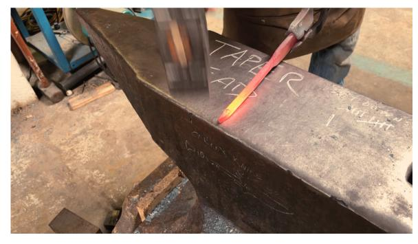
Step 6: Round the neck of the screwdriver. First knock down the corners and turn the stock from square to octagonal. Then knock down the remaining corners and turn the stock into a hexadecagon. Then hammer lightly while rotating the stock to make it round
