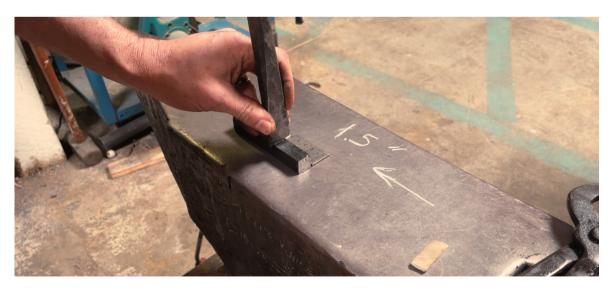
Step 2: At the 1.5" make use a spring fuller or top and bottom fullers and fuller the material down to 1/4" on all four sides.
