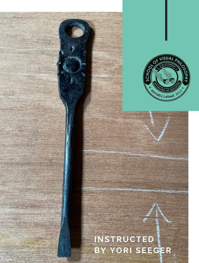
Step 1: Start this project off with a 4" piece of 5/8 square stock and make a mark 1.5" in from one side. This section will become the neck and flathead portion of the screwdirver.
