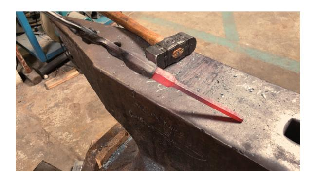
Step 4: Start working on the handle and draw the other end of the work down to 1/4" by 1"
