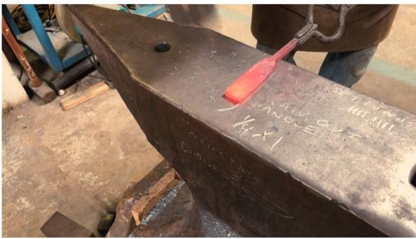
Step 5: Taper the 1/4" by 1/4" end to create the flathead portion of the screwdriver
