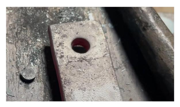
Step 8: Drift the hole to a 3/4" opening. Start with a 3/8" and proceed through 1/2", 5/8" and finally 3/4".
