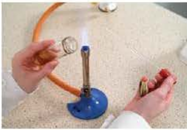
Figure 3.6 The neck of a glass container of a microbial culture is sterilised by passing it through the flame of a Bunsen burner without letting it get red hot. Notice that the scientist has the cap of the container in the crook of her little finger. This is a skill you must practise
