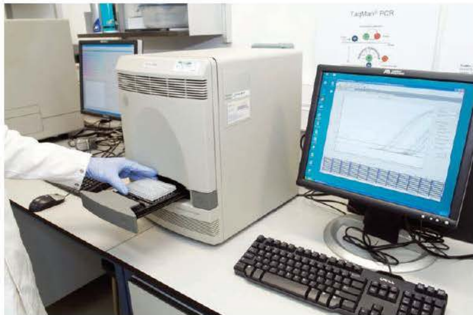
Figure 7.3 Loading a PCR machine. This demonstrates how much of the laboratory work involved in molecular genetics has become automated. The scientist has loaded the contents of each tube. Her next direct involvement will be to interpret the computer printout
